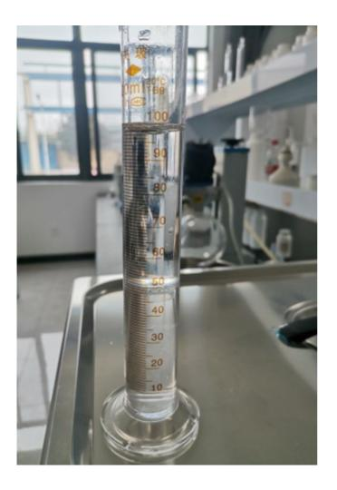
Throughout the mixing process, neither emulsification nor significant volume changes in either of the 50 mL samples were observed. Even after vigorous mixing, the two substances were able to quickly separate without evident mutual solubility.
